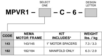
\*NOTE: Kit also includes Gasket, and Plugs for gauge, suction and case drain ports.
