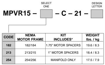
\*NOTE: Kit also includes Gasket, and Plugs for gauge, suction and case drain ports.
